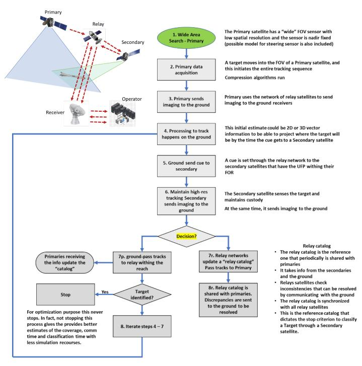
In the figure above, the flow of information is depicted during detection and classification when the intensive part of computation is performed on the ground.
