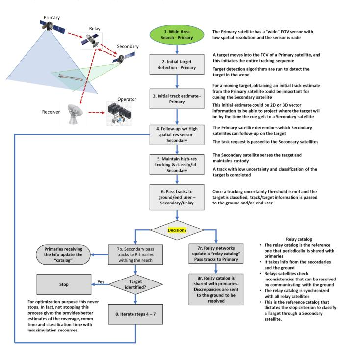
In the figure above, the flow of information is depicted during detection and classification when the intensive part of computation is performed on the satellites.
